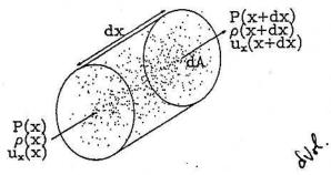
in dt, the mass flowing into the cylinder  $=\left[\rho(x)\left\{u_x(x)\right]dA\,dt\right]$  out of the cylinder  $=\left[\rho(x+dx)u_x(x+dx)\right]dA\,dt$ .
