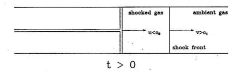
The shocked gas is heated, may be dissociated (if the ambient gas is molecular), and has sound speed
