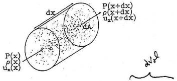
in dt, the momentum flowing into the cylinder  $= \rho(x)u_x(x) \cdot [u_x(x) \cdot dA \, dt]$  out of the cylinder  $= \rho(x+dx) \, u_x(x+dx) \cdot [u_x(x+dx) \cdot dA \, dt]$ .
