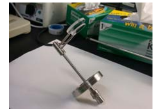
Figure 11. SXR lollipop device, featuring windows made of UV-fused silica (transmission cuts off abruptly above 7.3 eV), and sapphire (transmission cuts off above 8.3 eV). After the device was inserted into SSX, the windows were oriented at 90 degrees with respect to one another. Rotating the device then allowed us to position either window in the SXR line of sight.
