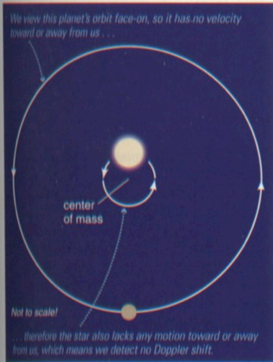
**a** If we view a planetary orbit face-on, we will not detect any Doppler shift at all.
