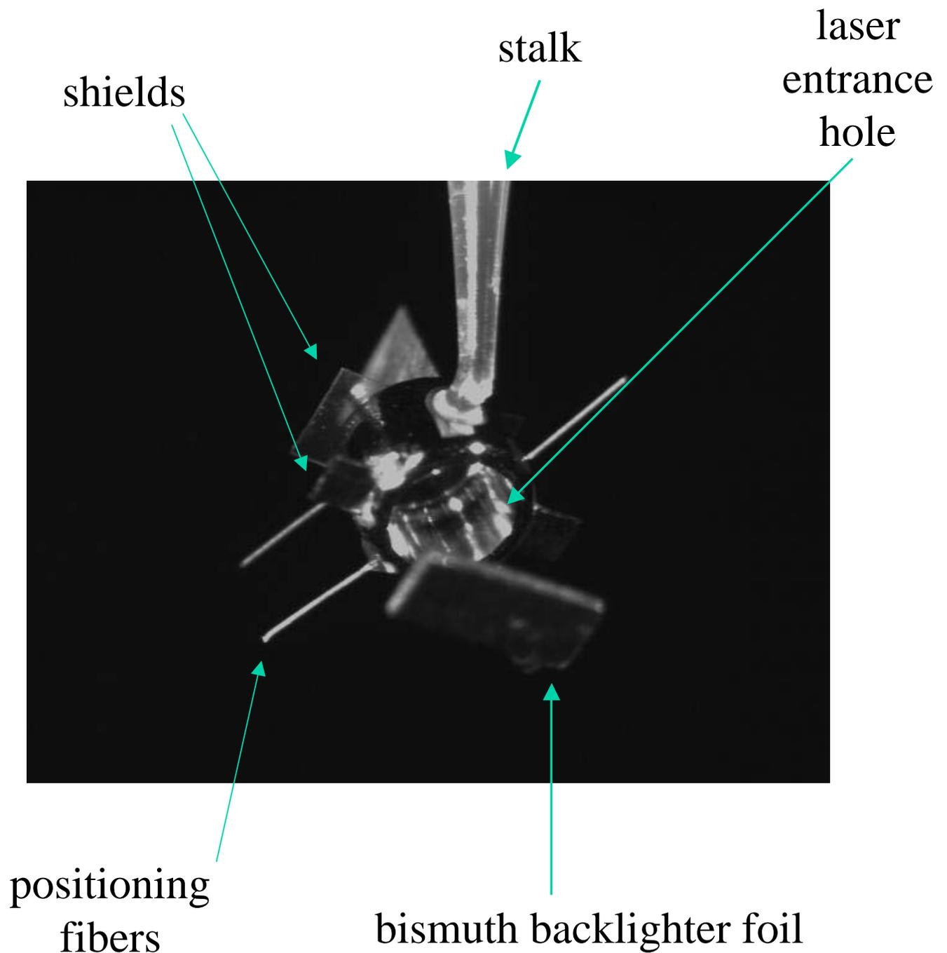
The ablator patch is mounted on the back of the hohlraum. The positioning fibers allow us to properly align the hohlraum in the OMEGA target chamber. This hohlraum is a
