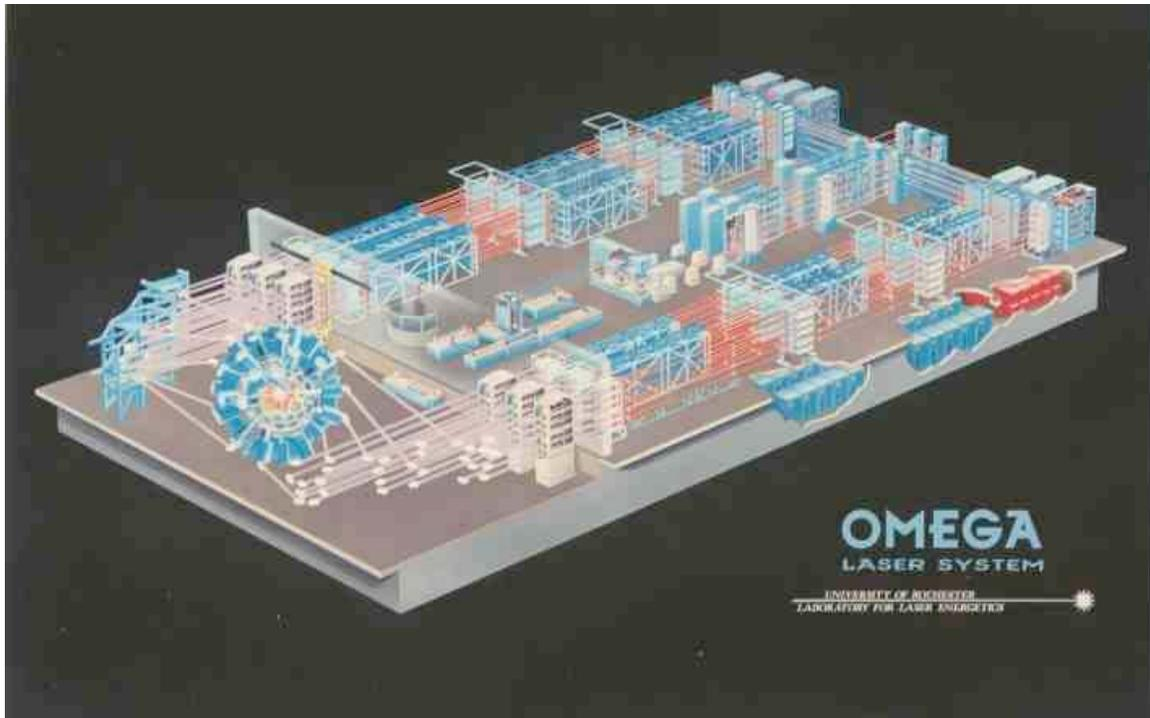
A Nd glass laser produces 60 beams of IR light, which are frequency-tripled into the ultraviolet. The total energy is 30 kJ, which can be delivered to a spot as small as 50 microns square in the target chamber (below) in less than 1 ns, for a total power of tens of terawatts, and a flux of  $10^{18}$  W/cm<sup>2</sup>.
