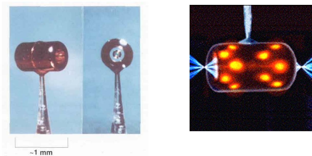
Images of a gold hohlraum used at the NOVA laser at Livermore. The picture on the right was taken in X-rays and shows the laser hotspots on the *interior* of the hohlraum radiating through the hohlraum walls.
