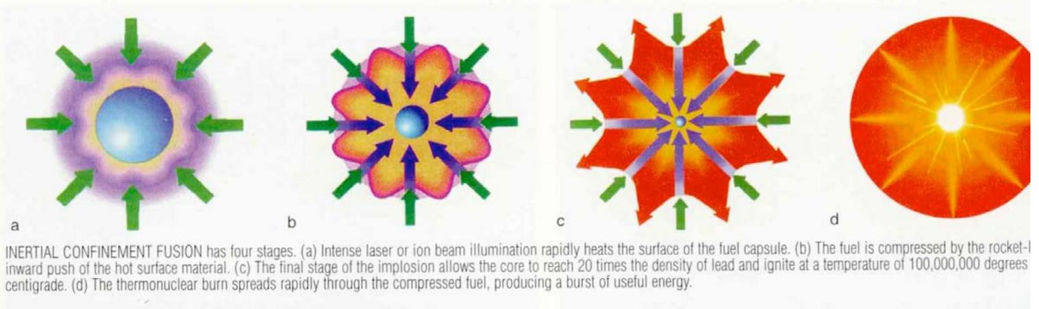
A spherical capsule filled with fuel (deuterium and tritium— isotopes of hydrogen) is bombarded with energy, *compressing* and *heating* a small region in the center of the fuel to values that allow the electrostatic repulsion of the nuclei to be overcome.
