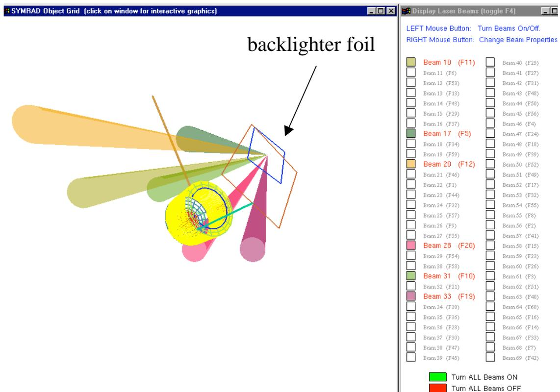
The chlorine spectral features are best seen in *absorption*, so we need a strong source of continuum X-rays to be absorbed by the chlorine in the tracer salt. This is provided by diverting several laser beams onto a bismuth ( $Z=83$ ) foil, referred to as the
