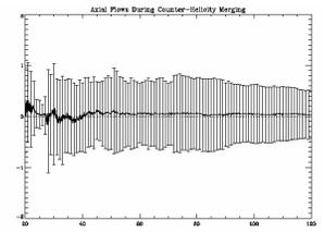
Figure 11b. Mean axial flow at the midplane for merging spheromaks, consistent with stagnation (v = 0).
