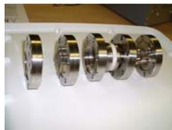
Figure 9. SXR filtered diode array.
