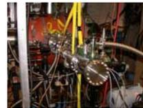
Figure 8. 0.2 m VUV monochromator on SSX.
