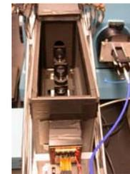
Figure 12. IDS output optics and multi-anode PMT array (bottom).
