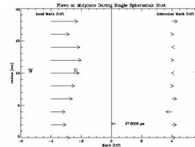
Figure 10b. High velocity axial flow with single spheromak (v = 100 km/s)
