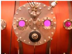
Figure 3. Plasma discharge in SSX (H plasma). Soft x-ray array is depicted (top).
