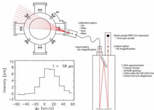
Figure 4. The SSX IDS setup. Typical low flow data.
