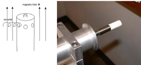
Figure 5. Mach probe schematic. Larger Mach II (top), smaller Mach I in He GDC plasma (bottom).
