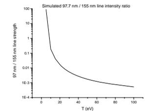
Figure 15. T<sub>e</sub> from CIII (97.7 nm) to CIV (155 nm) ratio (V. Chaplin, JP1.38).
