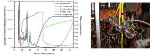
Figure 7. SXR filter response functions for photodiodes filtered by thin films of Al, Ti, Sn, and Zr
